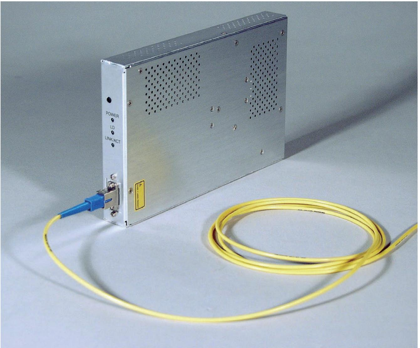
*Compact and High-performance OTDR Module for Optical Fiber Monitoring Systems*
